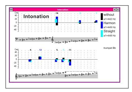
Intonation: The shifts of the resonance-peaks described above influence the intonation. The graph shows one example. In the lower register the trumpet with Wah-Wah mute is much sharper than the trumpet without mute (28 Cent above the values of the equal temperature scale instead of 10 Cent below). The mutes causes a shift not only to the individual resonances but also the intonation in general (which can be reduced with the main tuning slide).
